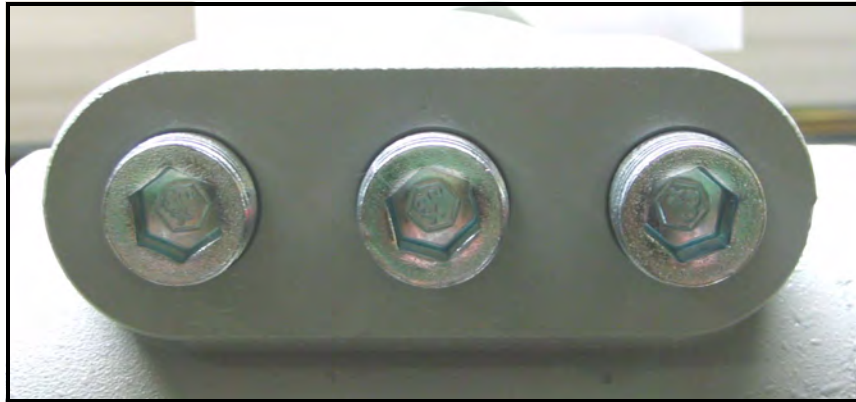
Figure 24: Conduit Inlet Ports
