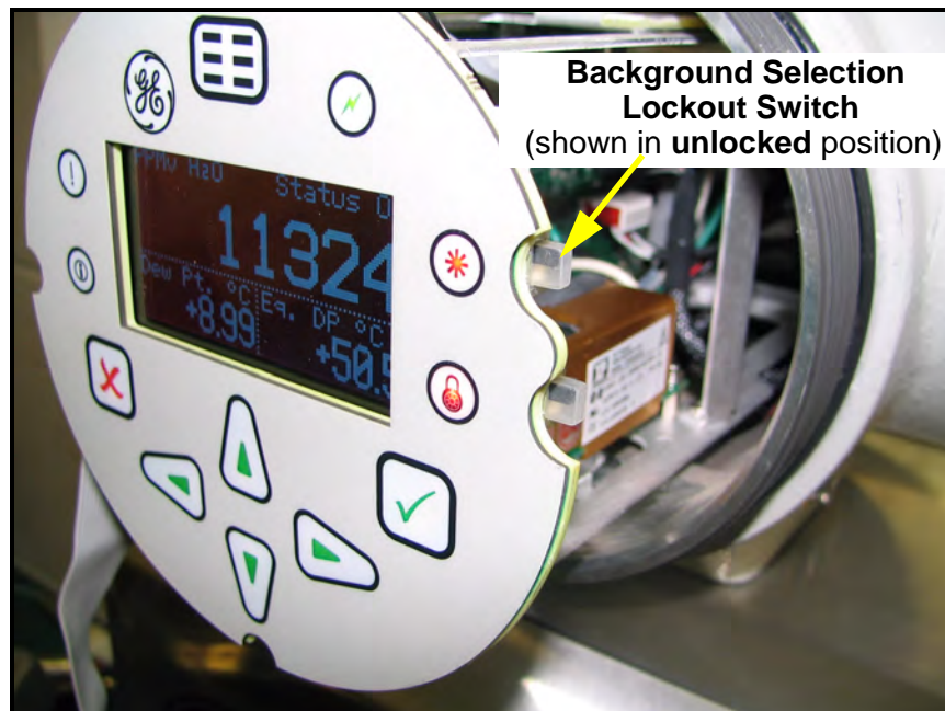
Figure 89: Background Selection Lockout Switch Location
